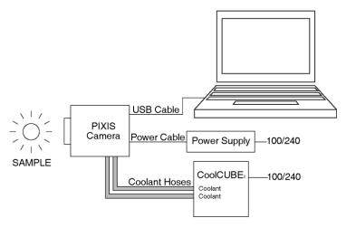
Figure 4. Typical Imaging Experiment Layout (Liquid-cooled Camera with CoolCUBE<sub>II</sub>)
